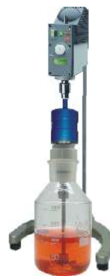
Magnetic drive coupled to 2 Ltr. glass vessel
